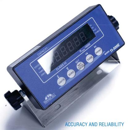
The TI-500E is a cost effective NTEP and Canadian certified digital indicator housed in a durable black ABS enclosure. It features a large easy to read green LED display and is capable of supporting up to four 350 ohm load cells through a junction box. The TI-500E allows for front panel access to the setup and calibration menu for simplified service and installation.
